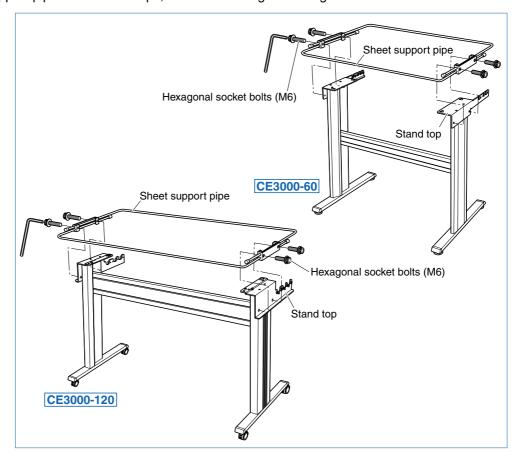
Mount the CE3000 cutting plotter on the stand by inserting the positioning pins on the stand into the positioning holes on the underside of the cutting plotter. Fasten using the four coin screws or hexagonal socket bolts (M6).
