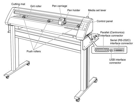
Cutting mat; Cutting or plotting is performed on this mat.Grit roller; Feeds the medium backward or forwardPush rollers; Pushes the medium against the grit rollersPen carriage; Moves the cutter pen to the left and rightPen holder; Holds the cutter pen and moves it up and down
