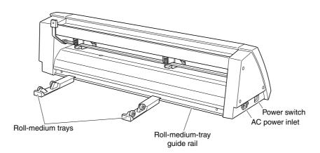
Roll-medium trays : Used to hold a roll medium
